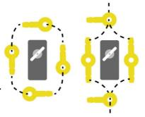
When putting a straw on the Strawbee on the servo motor horn, make sure to slide it over both the Strawbees and the motor arm itself. Encourage your students to pinch the end of the Straw first before sliding it so it covers both the servo horn and Strawbee.
